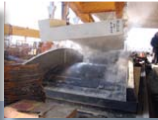
Precasters constructed the double-helix ramp at the center of the structure by creating custom forms that turned and sloped in precise configurations.
