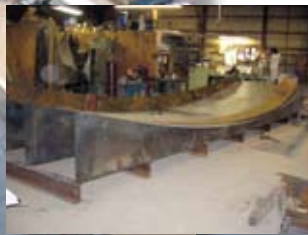
Precasters constructed the double-helix ramp at the center of the structure by creating custom forms that turned and sloped in precise configurations.
